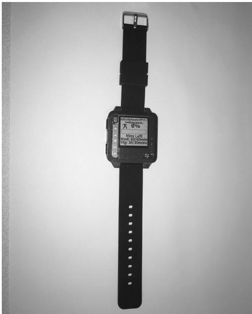
Figure 1. Image of the Amulet wearable device.
